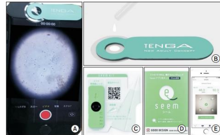
Fig. 4. Men's Loupe (Tenga Health Care) device and smartphone-based SEEM kit. (A) Men's Loupe 0.8 mm diameter ball lens microscope attached to smartphone. (B) Technique for loading semen sample into plastic jacket of ball lens microscope. (C) Magnifying lens semen analysis device with QR code sheet to download the application for operating. (D) Instructions of kit for use. (E) Screenshot of sample test results with concentration and motility.
